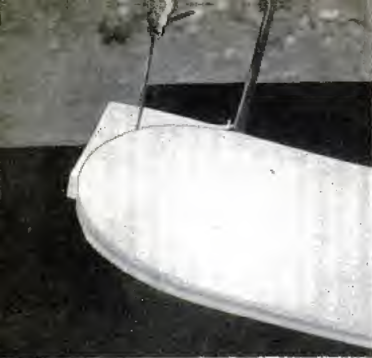
The rounded front of the skis is cut with a coping saw after 6-in. radius has been marked from pattern
